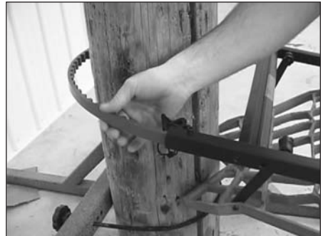
Step 7: Insert the belt back into the tube. NOTE: WARNING- point of arrow marks the end of the belt. No part of the arrow should be showing after the cams are engaged. Failure to follow these instructions could cause belt to disengage and cam to open. Now re-attach the cams firmly.
