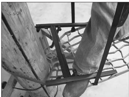
Step 3: Place your feet under the hinges and the bar as shown. Apply slight pressure to the hinge with the inside of the foot.
